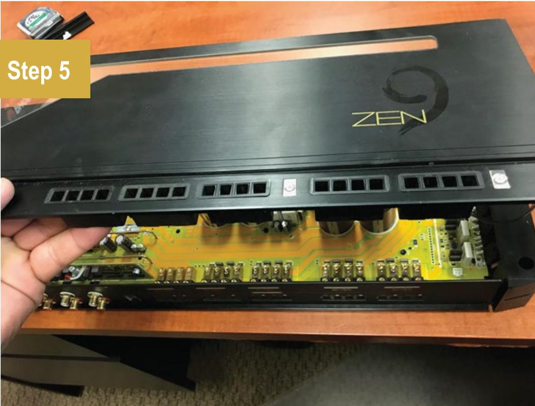
Lift in a pendulum motion from the front up to swing the top cover off of the amplifier
