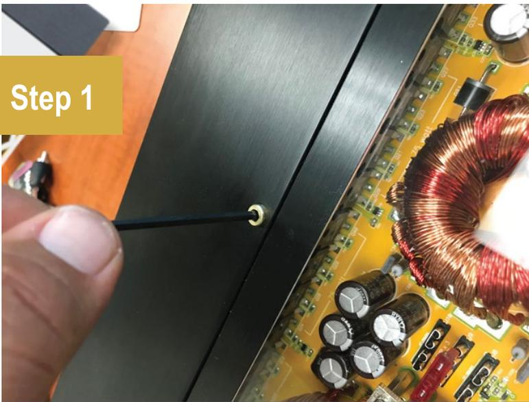
Remove the (5) 3mm hex head screws from the top of the amplifier
