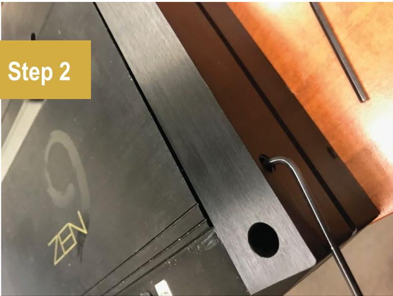
Remove the 2 top 2.5mm hex head from the end caps (ONLY REMOVE THE TOP SCREWS)
