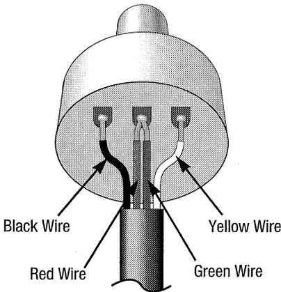
This diagram is provided to assist the custom installer with non-standard installs. **Note:** Swapping the black and yellow wires allows the knob to operate backwards (turn counter-clockwise to increase level, clockwise to decrease it).
