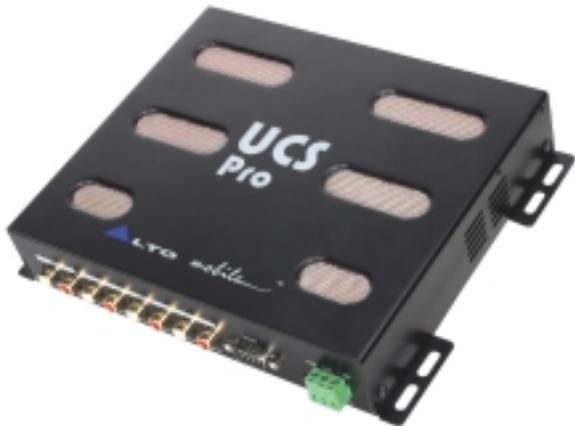
**UCS PRO** (Ultimate Control System) is an incredibly powerful 3-way 2 input / 6 Output audio system control center. The **UCS PRO's** 40-bit internal processing provides input / output gain control, a digital crossover with multiband EQ, time alignment and dynamic level control. **UCS PRO** also offers 24-bit A-D and D-A conversion with 48kHz sampling. All functions may be adjusted using **ALTO Mobile™ PC Editor** software, (supplied) and available as a free download.
