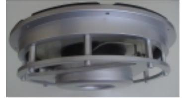
**Alto Mobile™** has continued their technological innovation in the **Falstaff** Line of Subwoofers. They feature a very slim profile thanks to their flat membrane and unique mechanical configuration that houses both the magnet assembly and damper inside the voice coil. This compact package provides the opportunity to install **Falstaff** Subwoofers in previously unused spaces, such as behind the driver’s seat in pickup trucks!
